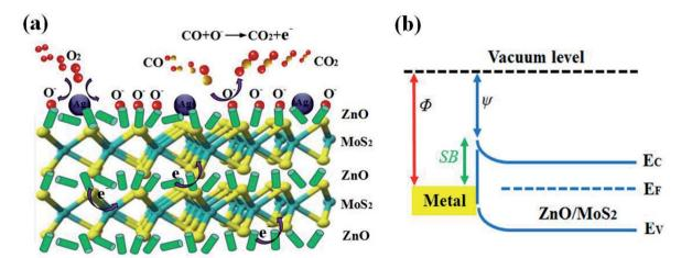
Fig. 12 (a) Schematic diagram of the Ag-ZnO-MoS<sub>2</sub> nanocomposite sensor towards CO gas; (b) energy band diagram of the Ag-ZnO-MoS<sub>2</sub> nanocomposite (reproduced from ref. 143 with permission from Elsevier).
