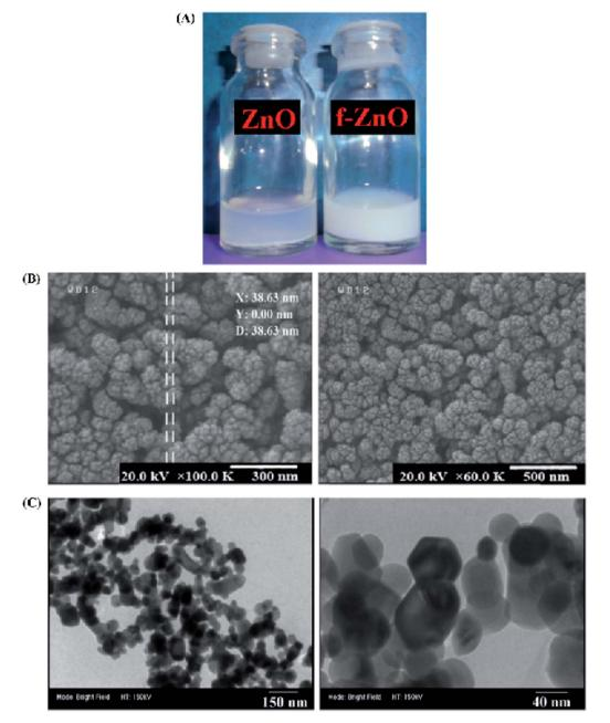
Fig. 8 (A) Photograph of aqueous dispersions of pure ZnO (left) and f-ZnO (right), and (B) FESEM and (C) TEM micrographs of f-ZnO (reproduced from ref. 104 with permission from Elsevier).
