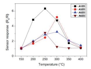
Fig. 13 Response of the Al-loaded and unloaded ZnO samples towards 50 ppm CO at different operating temperatures (reproduced from ref. 144 with permission from Elsevier).
