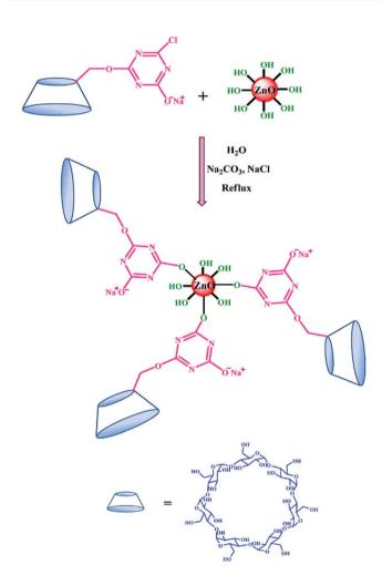
Fig. 7 Modification of ZnO nanoparticles with MCT- $\beta$ -CD (reproduced from ref. 104 with permission from Elsevier).
