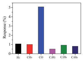
Fig. 11 Selectivity of the  $Ag-ZnO-MoS_2$  nanocomposite sensor towards 100 ppm gas species of  $H_2$ ,  $CH_4$ , CO,  $C_2H_2$ ,  $C_2H_6$  and  $C_3H_8$  (reproduced from ref. 143 with permission from Elsevier).
