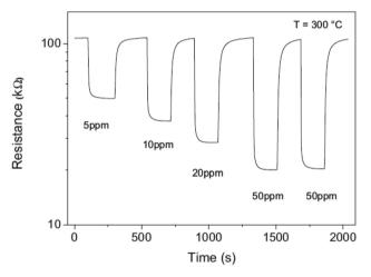
Fig. 15 Response of the A3ZO sensor as a function of CO concentration at 300 °C (reproduced from ref. 144 with permission from Flsevier)
