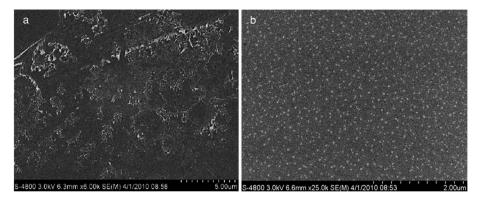
Fig. 6 FESEM of pure ZnO NPs (a) and grafted ZnO/polystyrene nanocomposite particles (b) dispersed in PVC matrices (reproduced from ref. 104 with permission from Elsevier).
