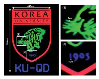
Fig. 6 Korea University logo fabricated using the QD-PR. For the KU logo, the minimum line width accomplished using the QD-PR was  $4-5\,$  um.
