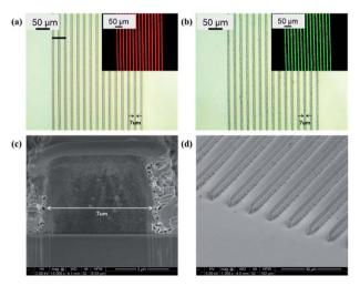
Fig. 4 Optical and fluorescence microscopy images (inset) of 7 μm line patterns of red (a) and green (b) QDs, respectively. Cross-sectional (c) and birds-eye view (d). SEM images of the photolithographic line pattern shown in (a) and (b).
