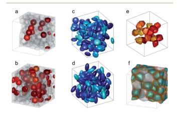
Fig. 14 Examples for the spatial distribution of nanoparticles with various shapes. (a and b) Spherical particles with different volume fractions. Reprinted figures with permission from Vivas *et al.*<sup>373</sup> Copyright 2020 by the American Physical Society. (c) and (d) Ellipsoids of revolution with different aspect ratios. (e) Clustered particles with polyhedron shapes. (f) A dense system of particles with a core–shell microstructure.
