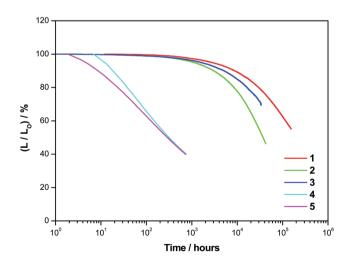
Fig. 9 Relative luminance,  $L/L_0$ , of vacuum-deposited devices based on **1–5** as a function of operation time projected at an initial luminance of 100 cd cm<sup>-2</sup>.
