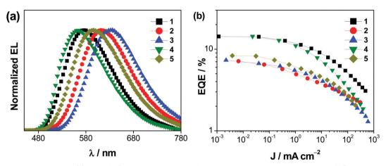
Fig. 8 (a) Normalized EL spectra and (b) plots of EQEs vs. current density of the vacuum-deposited devices based on 1–5.
