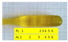
Fig. 1 Photograph of the GAGG:Ce,Mg crystal grown using the Czochralski method. Positions of plates used for characterization experiments (PL1-6) and compositional analysis (AL1-6) are indicated.
