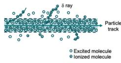
Fig. 1 Illustration of a heavy charged particle track showing the core (region of high ionization and excitation density) and penumbra (peripheral region where energy deposition occurs via  $\delta$  rays)
