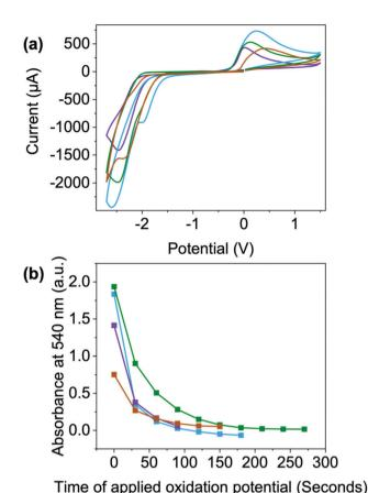
Fig. 7 (a) Cyclic voltammograms collected from buffered 10 mg mL $^{-1}$  solutions of NDI-I (—), NDI-V (—) adjusted to pH 9 and NDI-F (—) and NDI-GF (—) adjusted to pH 6 voltammograms measured in 1  $\times$  1 cm FTO windows. The scan rate of the cyclic voltammograms was 0.1 V s $^{-1}$ . (b) Time taken after the application of the oxidising potential for the absorption at 540 nm to return to 0.
