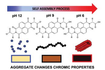
Fig. 1 Cartoon showing how an example NDI can have different aggregations depending on pH, ultimately effecting the colour of the reduced species in water
