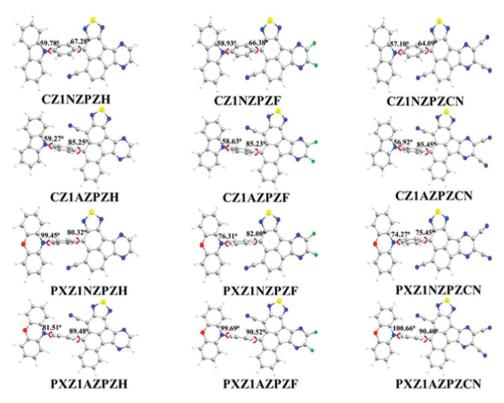
Fig. 1 Optimized geometries of newly designed molecules in the ground-state as obtained at  $\omega$ B97X/6-31G(d,p) level of theory.
