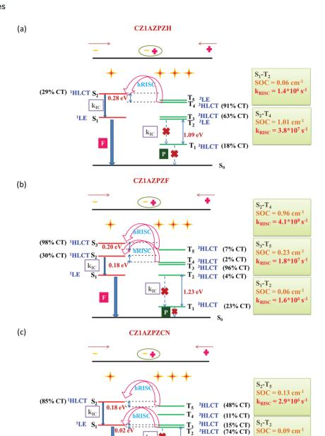
Fig. 5 Schematic depiction of a favourable hRISC process in (a) CZ1AZPZH, (b) CZ1AZPZF and (c) CZ1AZPZCN with the calculated energy levels, accompanying SOCs, and associated  $k_{RISC}$ .
