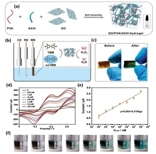
Fig. 8 (a) Schematic representation of the self-assembly of a GO/PVA/G4/H hydrogel. (b) Scheme of the GO/PVA/G4/H hydrogel as a working electrode to detect  $H_2O_2$ . (c) Photographs of the hydrogel before and after  $H_2O_2$  detection. (d) CV curves of the hydrogel. (e) The linear calibration plot for  $H_2O_2$ detection. (f) Photographs corresponding to the hydrogel sensor at different concentrations of H<sub>2</sub>O<sub>2</sub>.<sup>153</sup> Copyright The Royal Society of Chemistry 2020.
