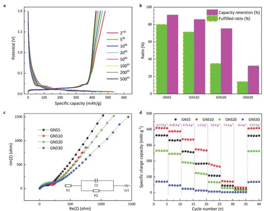
Fig. 4 (a) Discharge and charge patterns of GNS10 (0.17 A g<sup>-1</sup> within [0.05, 2] V), (b) capacity retention and fulfilled ratio of the cycling performance, (c) the galvano electrochemical impedance spectra of GNS5, GNS10, GNS20, and GNS30 from 10<sup>6</sup> to 0.01 Hz at AC = 0.1 mA with the inset equivalent circuit, and (d) rate capability of GNS5, GNS10, GNS20, and GNS30 at various current densities
