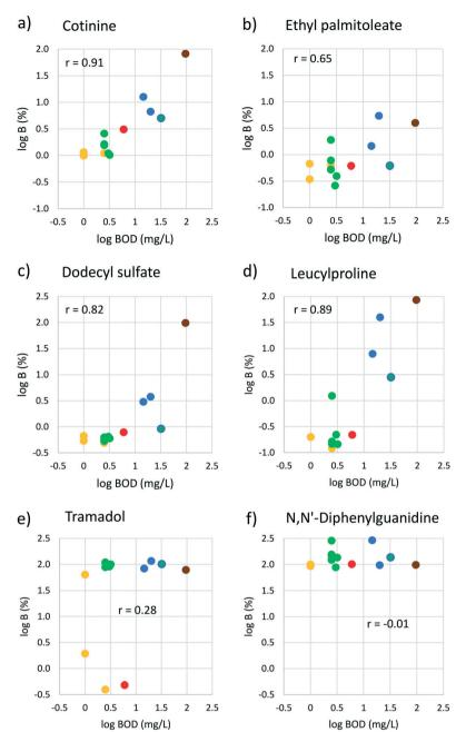
Fig. 4 log B versus log BOD plotted for 6 example chemicals. The correlation coefficient r is also shown. The colors indicate the treatmentstandard (see Table 1): red = ozonation; yellow = filtration; green = activated sludge with nitrification/denitrification; blue around green = biofilter/ activated sludge; blue = trickling filter; brown = primary treatment.
