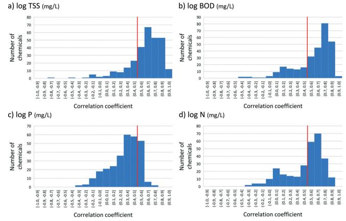
Fig. 3 Histograms of the correlation coefficient for 293 chemicals for the correlation of log B vs.: a) log TSS; b) log BOD; c) log P; d) log N in the effluent of 13 WWTPs. Bars to the right of the red line have a correlation coefficient <math>>0.5.
