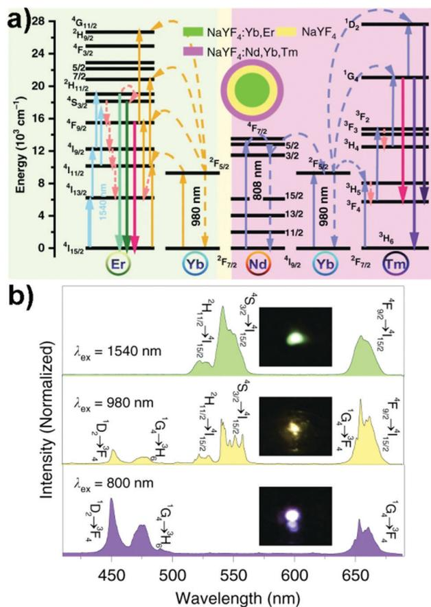
Fig. 2 (a) Proposed multiple excited state absorption and energy transfer mechanism in Nd<sup>3+</sup>, Yb<sup>3+</sup>, Er<sup>3+</sup>, and Tm<sup>3+</sup>-codoped UCNC.<sup>76</sup> (b) Upconversion emission spectra of UCNCs shown in (a) and the corresponding photo of UCNC films excited using λ<sub>ex</sub> = 800, 980 and 1540 nm laser excitation.<sup>76</sup> Reprinted with permission from ref. 76. Copyright 2020, Nature Publishing Group.
