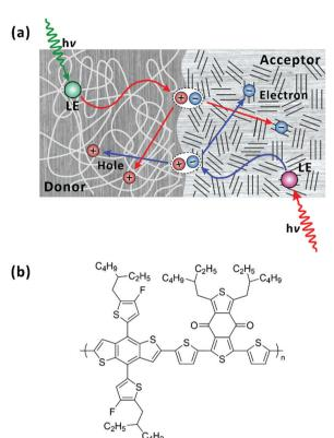
Fig. 1 (a) Simplified illustration of photophysical processes in bulkheterojunction organic photovoltaic devices. In both donor and acceptor domains, when locally excited (LE) states are generated upon photoexcitation, the LE states diffuse to the donor-acceptor interface and form charge-transfer state (CT). The CT state dissociates across the donoracceptor interface into charge-separated states. (b) Chemical structure of PM6
