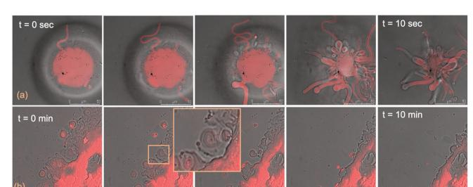
Fig. 8 CLSM images of AuNRs interacting with a GMO cubic film (overlay of fluorescence and transmission images): (a) disruption mechanism of a cubic film dewetted droplet by AuNRs, through the sequential extraction of lipid tubules from the bulk. (b) Mechanism of film excavation by AuNRs. Here, t = 0 corresponds to a lipid films/AuNRs incubation time  $\sim 0$  s, as the time needed for each image recording is less than 1 s.
