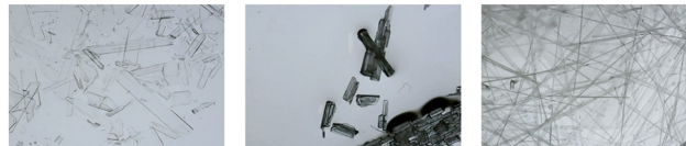
Fig. 6 Example images from each class in the experimental dataset, taken using the USB microscope on the screening robot. The images show examples of plates (left), blocks (centre) and needles (right).
