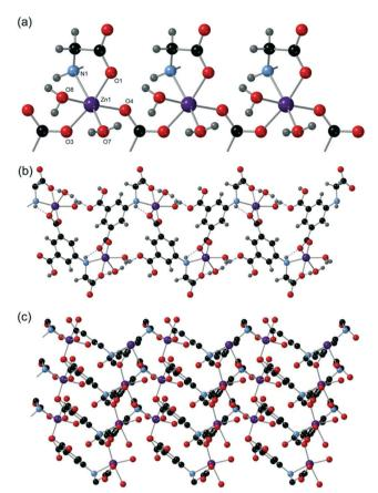
Fig. 11 The structure of compound 7 showing (a) a carboxylate-linked chain of Zn1 centres, (b) a corrugated two-dimensional sheet viewed side on and (c) a two-dimensional sheet viewed from the top (hydrogen atoms removed for clarity).
