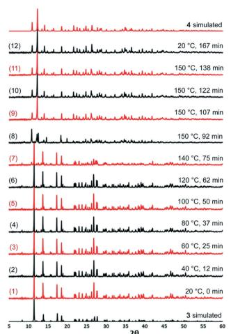
Variable temperature PXRD experimental results for 3 and 4.
