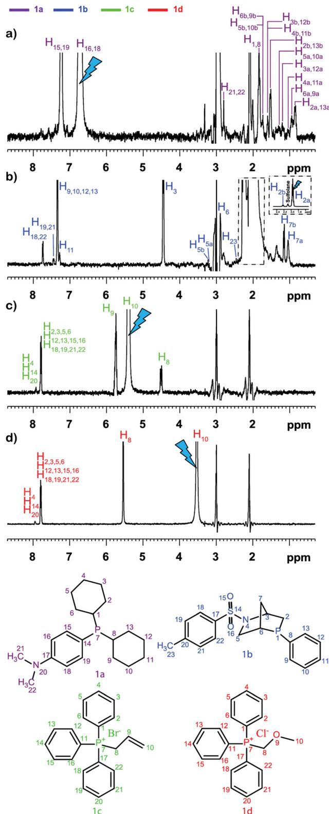
Fig. 4 Multiplet selective excitation 1D <sup>1</sup>H NOESY spectra of a phosphorus-based compound test mixture (20 mM) dissolved in sulfolane/DMSO-*d*<sub>6</sub> (7 : 3 v/v) (a–d), *t*<sub>m</sub> = 1 s, at 258 K, at 500 MHz (<sup>1</sup>H). The initial selective inversion pulses excite: (a) H<sub>16,18</sub>(1a), (b) H<sub>2a</sub>(1b), (c) H<sub>10</sub>(1c), and (d) H<sub>10</sub>(1d) proton resonances. Reproduced with permission from ref. 69, © 2020 American Chemical Society.
