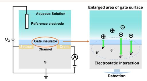
Fig. 10 Structure and principles of Bio-FETs.
