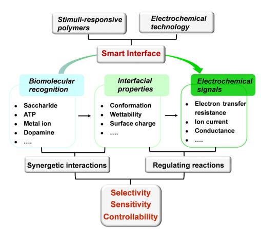
Fig. 1 Schematic illustration of the signal transduction for the electrochemical sensors based on stimuli-responsive polymers.
