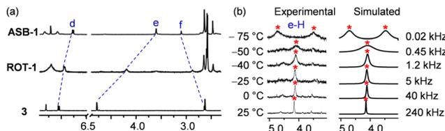
Fig. 5 (a) Partial  $^1\text{H}$  NMR ( $\text{CD}_2\text{Cl}_2$ , 400 MHz, 298 K) of **3**, **ROT-1** and **ASB-1**. (b) VT- $^1\text{H}$  NMR ( $\text{CD}_2\text{Cl}_2$ , 600 MHz) of **ROT-1** exhibiting the splitting of proton signal e-H into a 1:1 set and the corresponding rotational frequency at different temperatures.
