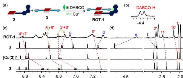
**Fig. 4** (a) Cartoon representation of the self-assembly of rotor **ROT-1** from four components. (b)  $(\text{CH}_2)_{\text{DABCO}}$  signal of **ROT-1** in the  $^1\text{H}$  NMR ( $\text{CD}_2\text{Cl}_2$ , 400 MHz). Partial  $^1\text{H}$  NMR ( $\text{CD}_2\text{Cl}_2$ , 400 MHz, 298 K) of **2**,  $[\text{Cu}(\mathbf{2})]^+$ , **3** and **ROT-1** in the (c) aromatic and (d) aliphatic region.
