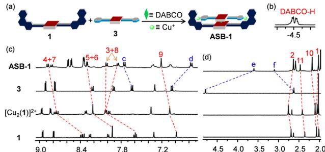
**Fig. 3** (a) Cartoon representation of the four-component self-assembly leading to the formation of **ASB-1**. (b) DABCO-H signal of **ASB-1** in  $^1\text{H}$  NMR ( $\text{CD}_2\text{Cl}_2$ , 400 MHz, 298 K). Partial  $^1\text{H}$  NMR ( $\text{CD}_2\text{Cl}_2$ , 400 MHz, 298 K) of **1**,  $[\text{Cu}_2(\mathbf{1})]^{2+}$ , **3** and **ASB-1** showing the (c) aromatic and (d) aliphatic region.
