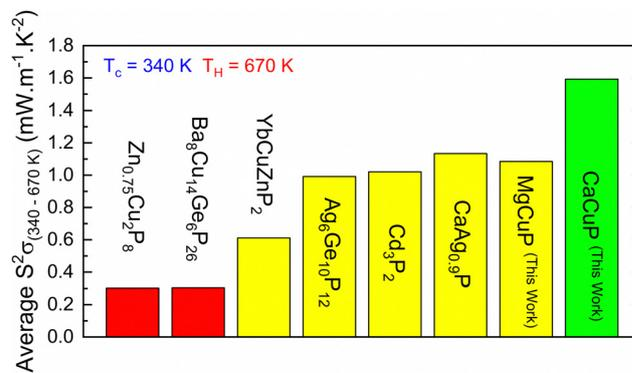
Fig. 4 Overview of temperature-average power factor ( $\langle S^2/\rho \rangle$ ) for leading metal phosphide thermoelectrics. Data taken from: Zn<sub>0.75</sub>Cu<sub>2</sub>P<sub>8</sub>,<sup>11</sup> Ba<sub>8</sub>Cu<sub>14</sub>Ge<sub>6</sub>P<sub>26</sub>,<sup>10</sup> YbCuZnP<sub>2</sub>,<sup>8</sup> Ag<sub>6</sub>Ge<sub>10</sub>P<sub>12</sub>,<sup>6</sup> Cd<sub>3</sub>P<sub>2</sub>,<sup>13</sup> CaAg<sub>0.9</sub>P,<sup>14</sup> MgCuP (This Work) and CaCuP (This Work).
