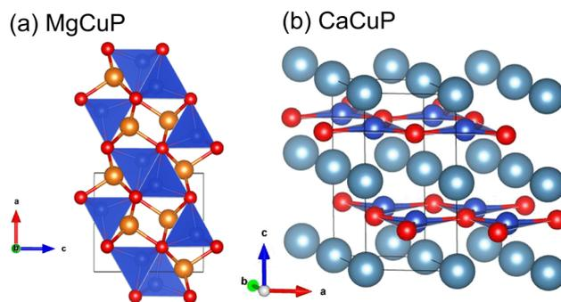
**Fig. 1** Crystal structures of (a)  $\text{MgCuP}$  and (b)  $\text{CaCuP}$ . Mg = orange, Ca = turquoise, Cu = blue and P = red. In  $\text{MgCuP}$ , edge linked  $\text{CuP}_4$  tetrahedra form chains aligned in the  $b$  direction.
