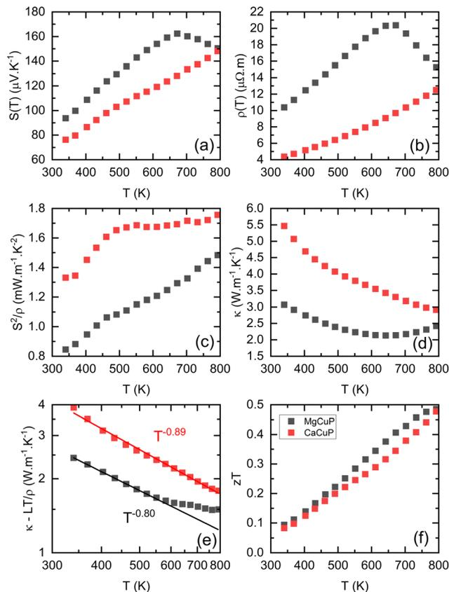
Fig. 2 Temperature dependence of (a)  $S(T)$ , (b)  $\rho(T)$ , (c)  $S^2/\rho(T)$ , (d)  $\kappa(T)$ , (e)  $\kappa_{\text{lat}}(T)$  and (f) the figure of merit,  $zT$  for MgCuP (black) and CaCuP (red) between 300–800 K.
