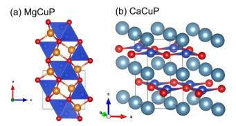
Fig. 1 Crystal structures of (a) MgCuP and (b) CaCuP. Mg = orange, Ca = turquoise, Cu = blue and P = red. In MgCuP, edge linked CuP<sub>4</sub> tetrahedra form chains aligned in the b direction
