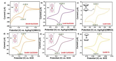
Fig. 2 Cyclic voltammograms for the reversible redox systems investigated with GC as the working electrode and Pt wire as the auxiliary electrode, measured at 100 mV s $^{-1}$ . (a) 30 mM Na[o-COSAN] in 0.3 M KNO<sub>3</sub>. (b) 1 mM Na[o-FESAN] in 0.3 M KNO<sub>3</sub>. (c) 1 mM FcMe in 0.3 M KNO<sub>3</sub>. (d) 5 mM Cs[o-COSAN] in 0.3 M TBAP/dry AcN. (e) 1 mM Cs[o-FESAN] in 0.3 M TBAP/dry AcN.
