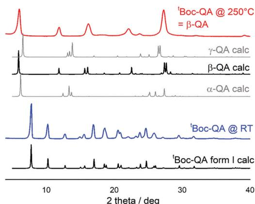
Fig. 2 Comparison of the experimental powder XRD patterns with those calculated on the basis of the single-crystal data for compounds.<sup>34</sup> Top: thermal deprotection of a polycrystalline sample of  $\epsilon$ -Boc-QA leads to formation of  $\beta$ -QA.
