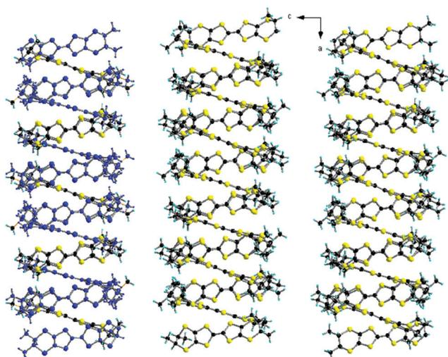
Fig. 3 Crystalline packing of [(*S*)-1]<sub>9</sub>(Mo<sub>6</sub>O<sub>19</sub>)<sub>5</sub>·(CHCl<sub>3</sub>)<sub>2</sub> in the *ac* plane with a highlight of the two types of donors (left column, the asymmetric unit contains two donors 1\*TTF + ½\*TTF). Anions and solvent have been omitted.
