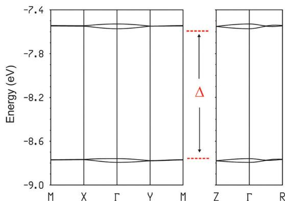
Fig. 11 Calculated three-dimensional band structure for the donor sublattice of [(rac)-1]<sub>2</sub>(Mo<sub>6</sub>O<sub>19</sub>), where  $\Gamma = (0, 0, 0)$ ,  $X = (a^*/2, 0, 0)$ ,  $Y = (0, b^*/2, 0)$ ,  $M = (a^*/2, b^*/2, 0)$ ,  $Z = (0, 0, c^*/2)$  and  $R = (a^*/2, b^*/2, c^*/2)$ .  $\Delta$  is the energy gap between the filled and empty bands.
