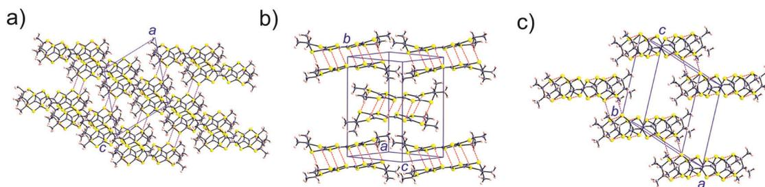
Fig. 10 Donor sublattice of the [(rac)-1]<sub>2</sub>(Mo<sub>6</sub>O<sub>19</sub>) salt. The S··S contacts shorter than 3.9 Å are shown as dashed red (intra-dimer) and purple (inter-dimer) lines.
