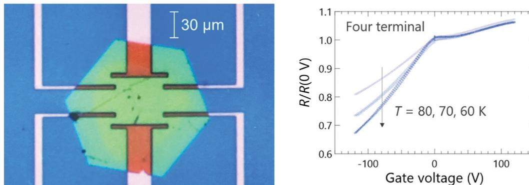
Fig. 9 Microscope image of the thin hexagonal crystal of [(S)-1]<sub>9</sub>(Mo<sub>6</sub>O<sub>19</sub>)<sub>5</sub>·(CHBr<sub>3</sub>)<sub>2</sub> attached on the SiO<sub>2</sub>/Si substrate with pre-patterned gold electrodes (left). Gate voltage dependence of normalized resistance of the crystal at selected temperatures of 60 K, 70 K, and 80 K (right).
