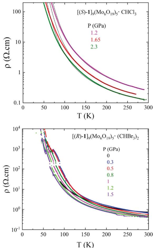
Fig. 5 Temperature dependence of the electrical resistivity  $\rho$  at different applied pressures for a single crystal of  $[(S)\text{-}1]_9(\text{Mo}_6\text{O}_{19})_5 \cdot (\text{CHCl}_3)_2$  (top) and for a single crystal of  $[(R)\text{-}1]_9(\text{Mo}_6\text{O}_{19})_5 \cdot (\text{CHBr}_3)_2$  (bottom).
