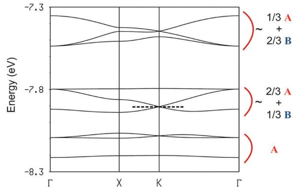
Fig. 7 Calculated band structure for the donor layers of  $[(S)\text{-}1]_9(\text{Mo}_6\text{O}_{19})_5 \cdot (\text{CHCl}_3)_2$  where  $\Gamma = (0, 0)$ ,  $X = (a^*/2, 0)$  and  $K = (a^*/3, a^*/3)$ . The dashed line indicates the highest occupied level assuming double occupation of the levels. The approximate composition of the bands is shown at the right hand of the diagram.
