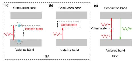
Fig. 6 Electronic transitions under fs laser excitation. (a and b) Saturable absorption (SA) is induced by single-photon absorption (SPA). (a) Excitonic absorption and (b) defect state absorption. (c) Reverse saturable absorption (RSA) is mainly induced by two-photon absorption (TPA).
