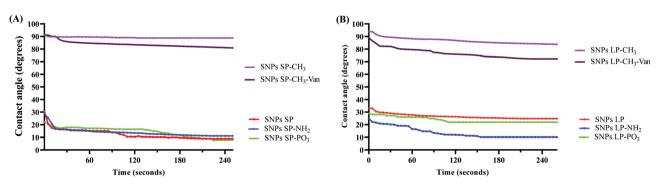
Fig. 3 Functionalisation of SNPs with octadecyl methyl groups reduced their hydrophilicity. (A) The change in contact angle for SNPs SP with/without various functional groups at different time intervals, showing increase of hydrophobicity in SNPs SP functionalised with octadecyl methyl groups. (B) The change in contact angle for SNPs LP with/without various functional groups at different time intervals, showing increase of hydrophobicity in SNPs LP functionalised with octadecyl methyl groups
