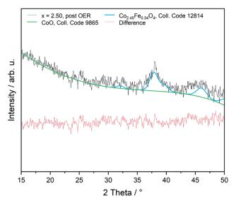
Fig. 8 Rietveld refinement of sample x = 2.50 on Si after OER measurement (GIXRD, 1°).
