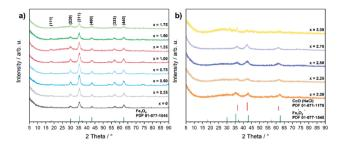
Fig. 1 PXRD patterns of (a)  $Co_xFe_{3-x}O_4$  (x=0-1.75) and (b)  $Co_x-Fe_{3-x}O_4$ /( $Co_{x/3}Fe_{(1-x)/3}$ )O (x=2-3) with references for  $Fe_3O_4$  (PDF 01-077-1545) and CoO (PDF 01-071-1178).
