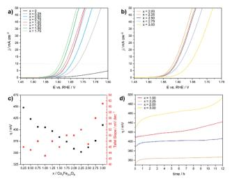
Fig. 4 Linear sweep voltammograms for (a)  $Co_xFe_{3-x}O_4$  (x=0-1.75) and (b)  $(Co_{x/3}Fe_{(1-x)/3})O$  ( $x \ge 2$ ) in 1 M KOH electrolyte with a scan rate of 5 mV s<sup>-1</sup>, (c) overpotential and Tafel slope *versus* the cobalt content and (d) chronoamperometry measurements at 10 mA cm<sup>-2</sup> (geometrical surface area).
