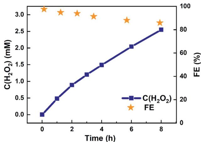
Fig. 3  $\text{H}_2\text{O}_2$  accumulation using 4 : 1 (Ti,Mn) $\text{O}_x$ -coated FTO electrode operated in the dark. Cumulative  $\text{H}_2\text{O}_2$  concentration and the respective cumulative FE vs. time. The electrode area was  $1.2 \text{ cm}^2$ , and the applied potential was  $+1.31 \text{ V}$  vs. Ag/AgCl (equivalent to an overpotential of  $150 \text{ mV}$ ) in a  $20 \text{ mL}$   $0.5 \text{ M}$   $\text{pH} = 7.0$  PB solution.
