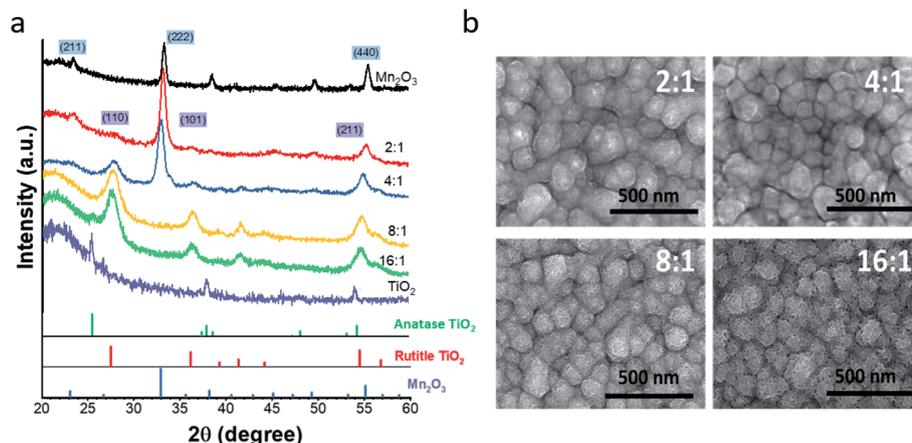
Fig. 1 (a) Grazing incident X-ray diffraction (GI-XRD) spectra and (b) plan-view scanning electron microscope (SEM) images of annealed (Ti,Mn) $O_x$ . Samples denoted  $Mn_2O_3$  and  $TiO_2$  represent annealed ALD  $MnO_x$  and  $TiO_x$ , respectively.
