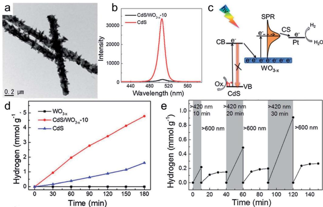
Fig. 9 TEM image (a) of CdS/WO<sub>3-x</sub> nanowires, PL spectra (b) of CdS/WO<sub>3-x</sub> and CdS, the photocatalysis mechanism (c) on plasmonic CdS/WO<sub>3-x</sub>. Photocatalytic hydrogen generation over CdS/WO<sub>3-x</sub> as catalysts under >420 nm (d) and >600 nm (e) light irradiation. Reproduced with permission from ref. 49. Copyright 2018, Elsevier B.V.
