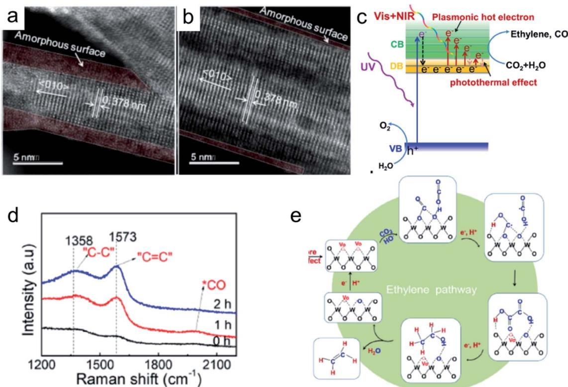
Fig. 10 TEM images of  $\text{WO}_{3-x}$  nanowires with thick (a) and thin (b) amorphous layers, and their photocatalytic mechanism (c) for  $\text{CO}_2$  reduction. Raman spectra (d) and possible ethylene generation pathway (e) over  $\text{WO}_{3-x}$  nanowires with thin amorphous layer as catalysts during  $\text{CO}_2$  photocatalytic reduction. Reproduced with permission from ref. 109. Copyright 2020, Elsevier B.V.
