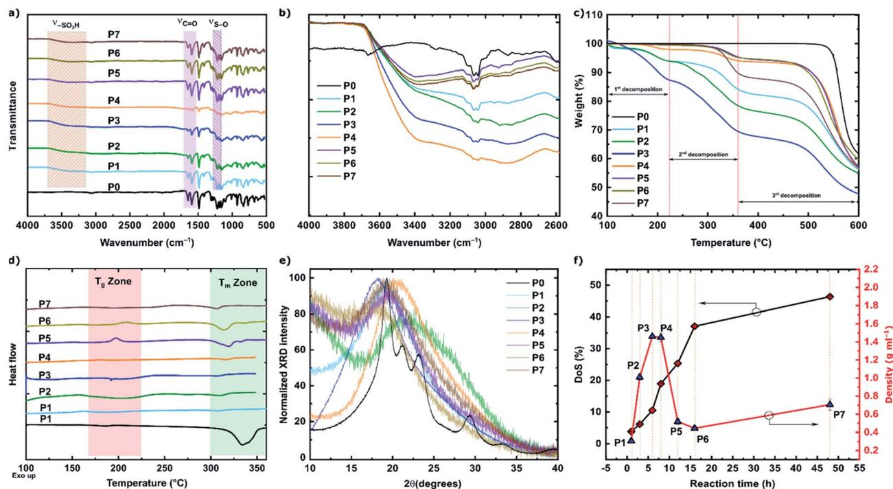
Fig. 2 SPEEK characterization: FTIR spectra in the range of (a) 500–4000  $\text{cm}^{-1}$  and (b) 2600–4000  $\text{cm}^{-1}$ ; (c) thermal degradation obtained using TGA; (d) DSC thermograms at 100–350  $^\circ\text{C}$ ; (e) WAXD spectra with  $2\theta = 8\text{--}40^\circ$ ; and (f) DoS and densities of polymers as a function of the sulfonation reaction time.
