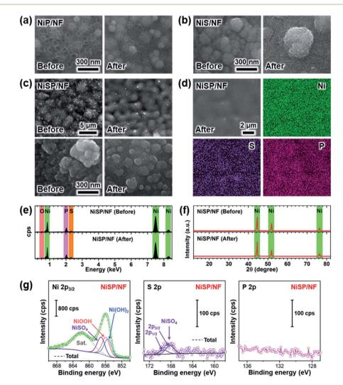
Fig. 6 OER electrochemical post analysis results: SEM images before and after the OER for (a) NiP, (b) NiS and (c) NiSP films, (d) elemental mapping after the OER, (e) EDX spectra and (f) XRD comparison for NiSP film, (g) XPS post analysis.
