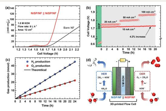
Fig. 8 Overall water splitting results: (a) i-V curves, (b) chronopotentiometric run at different current densities for 20 h, (c) gas evolution measurements at 10 mA cm<sup>-2</sup>, and (d) schematic illustration of the assembled flow cell with NiSP/NF electrodes using 1 M KOH electrolyte.
