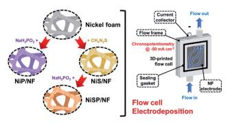
Fig. 1 Schematic illustration of the flow electrodeposition approach using a 3D-printed flow cell.
