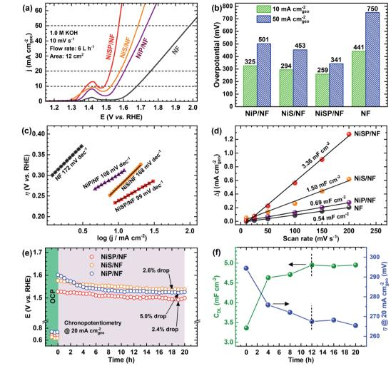
Fig. 4 OER electrochemical characterization results: (a) anodic i-V curves, (b) overpotentials at 10 and 50 mA cm<sup>-2</sup>, (c) Tafel slopes, (d) doublelayer capacitances and (e) chronopotentiometric runs at 20 mA cm<sup>-2</sup> during a period of 20 h, using the as-prepared electrodes in 1 M KOH electrolyte. (f) Double layer capacitance and overpotential at 20 mA cm<sup>-2</sup> of the NiSP/NF electrode with time.
