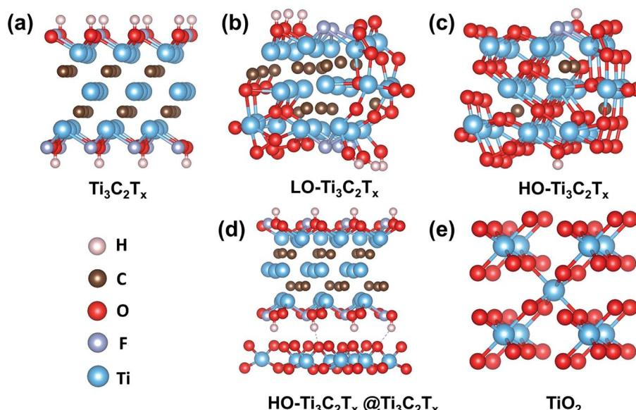
Fig. 5 Predicted crystal structures of Ti<sub>3</sub>C<sub>2</sub>T<sub>x</sub>, LO-Ti<sub>3</sub>C<sub>2</sub>T<sub>x</sub>, HO-Ti<sub>3</sub>C<sub>2</sub>T<sub>x</sub>, HO-Ti<sub>3</sub>C<sub>2</sub>T<sub>x</sub>@Ti<sub>3</sub>C<sub>2</sub>T<sub>x</sub> and TiO<sub>2</sub> carried out by VASP code based on DFT.
