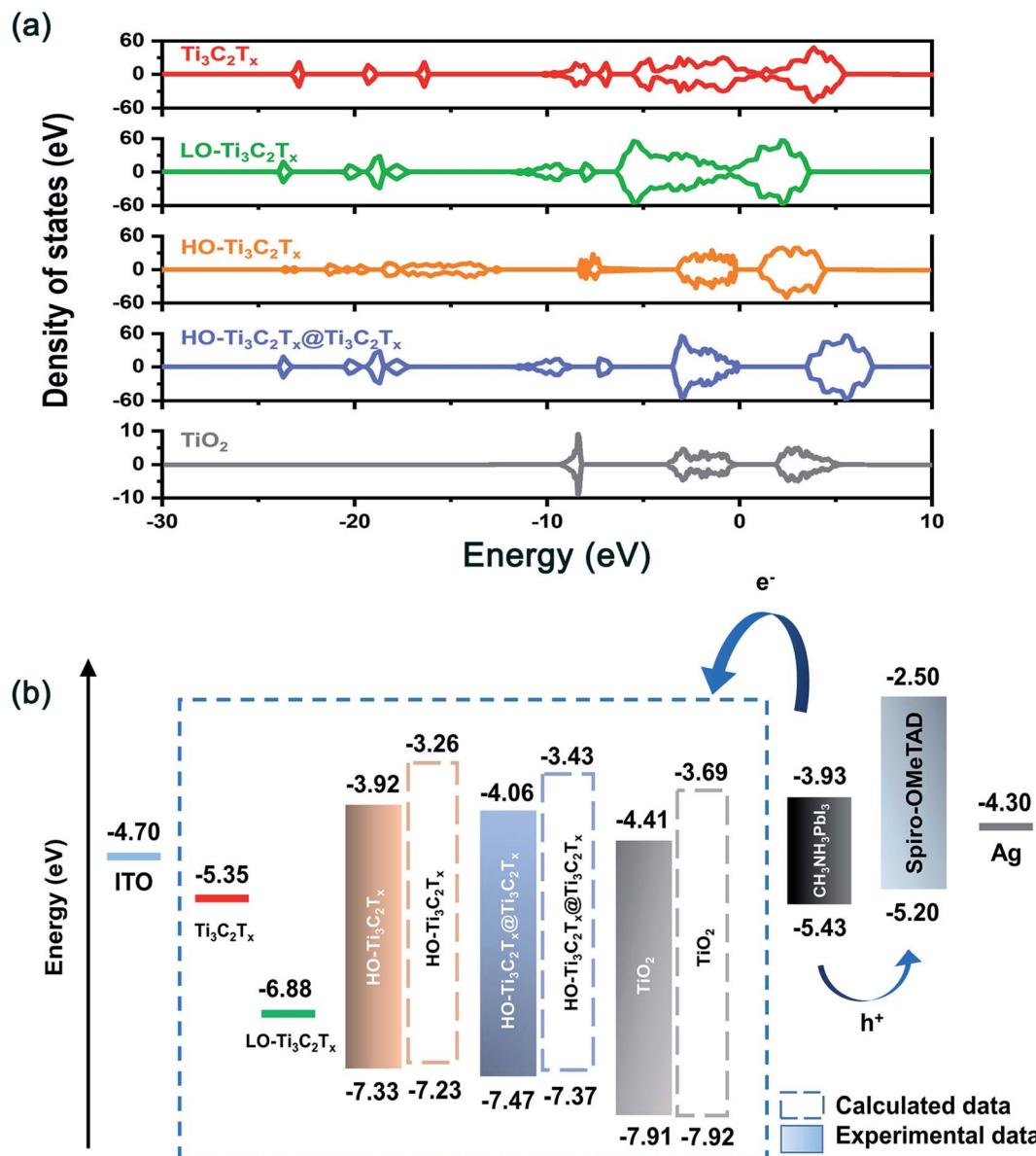
Fig. 6 (a) Calculated density of states for  $\text{Ti}_3\text{C}_2\text{T}_x$ ,  $\text{LO}-\text{Ti}_3\text{C}_2\text{T}_x$ ,  $\text{HO}-\text{Ti}_3\text{C}_2\text{T}_x$ ,  $\text{HO}-\text{Ti}_3\text{C}_2\text{T}_x@\text{Ti}_3\text{C}_2\text{T}_x$ ,  $\text{TiO}_2$  and (b) schematic diagram of devices' each layer based on different ETLs determined by DFT calculation and UPS data.
