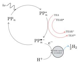
Fig. 9 Example of a possible catalytic cycle in the presence of a noble metal co-catalyst.
