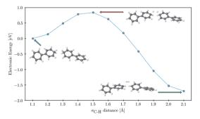
Fig. 7 Predicted energy profile for the H<sub>2</sub> formation step showing the energy of each geometry along the constrained optimization scan. All values calculated with B3LYP/cc-pVTZ in combination with a water solvation model and provided relative to the starting point of two PP2-H' molecules.
