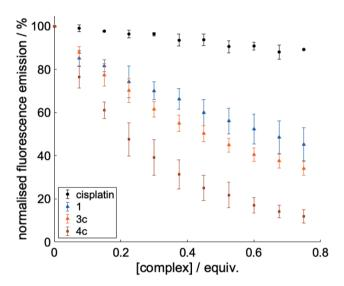
Fig. 4 Normalised fluorescence emission of the Tyr10 residue of A $\beta$ 1-16 on addition of cisplatin (negative control), 1, 3c and 4c (0 to 0.75 eq., phosphate buffer, pH 7.4). Quenching is observed with both square planar 1 (blue) and octahedral 3c and 4c (orange) complexes. The highest degree of quenching is seen with Co-salnaph complex 4c (square). All data is reported as the mean  $\pm$  standard deviation of three independent experiments.
