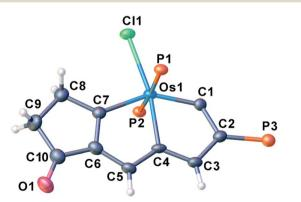
Fig. 1 X-ray crystal structure of the cation of 1 (thermal ellipsoids are set at the 50% probability level and the phenyl groups in the PPh<sub>3</sub> moieties are omitted for clarity). Selected bond lengths [Å] and angles [°]: Os1–C1: 1.858(3), Os1–C4: 2.106(3), Os1–C7: 2.045(3), C1–C2: 1.398(4), C2–C3: 1.398(5), C3–C4: 1.398(5), C4–C5: 1.397(5), C5–C6: 1.410(5), C6–C7: 1.396(5), C4–Os1–C1: 72.31(13), C7–Os1–C4: 75.01(13).
