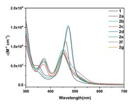
Fig. 6 UV-Vis spectra of osmapentalyne 1 and its *N*-functionalized derivatives 2a-2g (CH<sub>2</sub>Cl<sub>2</sub>, rt,  $5.0 \times 10^{-5}$  M).
