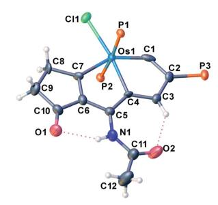
Fig. 3 X-ray crystal structure of the cation of 2c (thermal ellipsoids are set at the 50% probability level and the phenyl groups in the PPh<sub>3</sub> moieties are omitted for clarity). Selected bond lengths [Å] and angles [°]: Os1–C1: 1.818(10), Os1–C4: 2.146(7), Os1–C7: 2.057(8), C1–C2: 1.411(12), C2–C3: 1.415(11), C3–C4: 1.394(10), C4–C5: 1.411(11), C5–C6: 1.427(11), C6–C7: 1.356(11), C5–N1: 1.387(11), N1H···O1: 2.107, H3···O2: 2.105 C4–Os1–C1: 72.6(3), C7–Os1–C4: 75.7(3).
