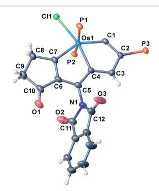
Fig. 2 X-ray crystal structure of the cation of 2a (thermal ellipsoids are set at the 50% probability level and the phenyl groups in the PPh<sub>3</sub> moieties are omitted for clarity). Selected bond lengths [Å] and angles [°]: Os1–C1: 1.842(2), Os1–C4: 2.111(2), Os1–C7: 2.044(2), C1–C2: 1.404(3), C2–C3: 1.404(3), C3–C4: 1.414(3), C4–C5: 1.397(3), C5–C6: 1.397(3), C6–C7: 1.388(3), C5–N1: 1.430(3), C4–Os1–C1: 72.32(9), C7–Os1–C4: 75.89(9).
