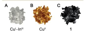
Fig. 1 Photographs of crystals of (A) the colorless double perovskite,  $(PEA)_4Cu^I | n^{III}Cl_8$ , (B) the yellow single perovskite,  $(PCA)_2Cu^I | Cl_4$ , and (C) the black perovskite,  $(BA)_4[Cu^I | (Cu^I | n^{III})_{0.5}Cl_8]$  ( $1_{BA}$ ), featuring a 1 : 1 blend of the inorganic lattices in A and B. The black color arises from  $Cu^{+/2+}$  mixed valency. PEA = phenethylammonium, PCA = p-chloroanilinium, and BA = butylammonium.
