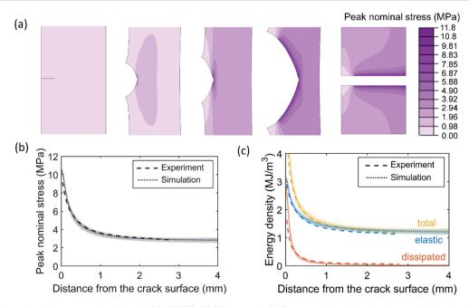
Fig. 5 FE simulation of crack propagation in the EA0.2-0.05(2.61) SEN sample. (a) Contour of peak nominal stress before, during and after crack propagation. (b and c) Comparison between simulation results and experimental data in terms of (b) the peak nominal stress and (c) the total, elastic and dissipated energy densities in the completely fractured SEN sample. The shaded regions represent ranges of the simulation results and the dotted lines represent the averages of simulation results.
