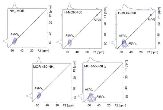
Fig. 3  $^{27}$ Al MQMAS NMR spectra measured under ambient conditions for NH<sub>4</sub>–MOR, H–MOR-450, H–MOR-550, MOR-450-NH<sub>4</sub> and MOR-550-NH<sub>4</sub>. The F1 projection shows a purely isotropic dimension and the F2 projection depicts the corresponding  $^{27}$ Al MAS NMR spectrum, which is acquired in a separate experiment.
