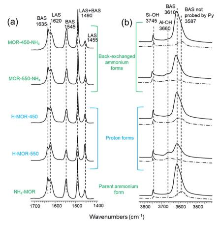
Fig. 4 FTIR spectra of (a) adsorbed pyridine over activated  $NH_4$ -MOR, H-MOR-450, H-MOR-550, MOR-450-NH<sub>4</sub> and MOR-550-NH<sub>4</sub>; (b) samples activated under vacuum at 450 °C for 4 h (solid line) and after pyridine adsorption-desorption at 150 °C (dashed line) in the OH stretching region. The names of the samples refer to the form of the zeolite prior to heat treatment in the IR setup.
