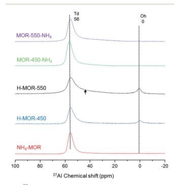
Fig. 2  $^{27}$ Al MAS NMR spectra of zeolite MOR under ambient conditions of NH<sub>4</sub>–MOR, H–MOR-450, H–MOR-550, MOR-450-NH<sub>4</sub> and MOR-550-NH<sub>4</sub>. The broad shoulder at the high field side of the peak corresponding to tetrahedrally coordinated framework aluminum in H–MOR-550 is highlighted by the black arrow mark.
