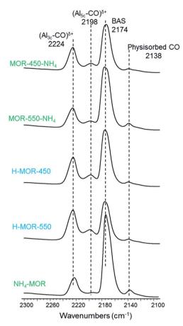
Fig. 5 FTIR spectra of adsorbed carbon monoxide over activated parent ammonium form NH<sub>4</sub>–MOR, H–MOR-450, H–MOR-550, MOR-450-NH<sub>4</sub> and MOR-550-NH<sub>4</sub>. The names of the samples refer to the form of the zeolite prior to heat treatment in the IR setup.
