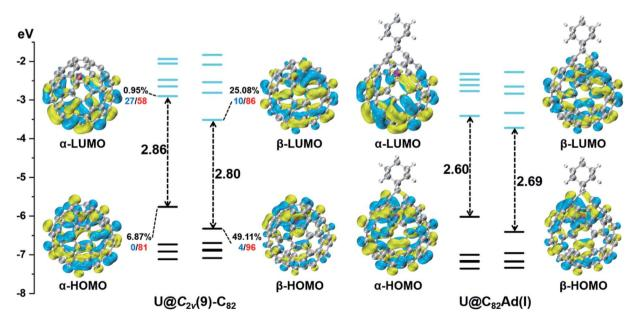
Fig. 11 Frontier molecular orbitals of  $U@C_{2v}(9)-C_{82}$  and  $U@C_{2v}(9)-C_{82}Ad(I)$  (occupied: black; unoccupied: cyan). For selected orbitals, the participation (%) of the U AOs is first given, followed by two numbers showing the % contribution of the U-5f (red), or -6d (blue) AOs to this metal hybrid orbital.
