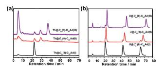
Fig. 5 (a) HPLC traces of isomerization of Th@ $C_{3v}$ (8)- $C_{82}$ Ad(I, II, III) and (b) recycling HPLC traces of isomerization of U@ $C_{2v}$ (9)- $C_{82}$ Ad(I, II, III) at room temperature. HPLC conditions: Buckyprep column (10 mm  $\times$  250 mm); flow rate, 4 mL min $^{-1}$ ; toluene as the mobile phase.
