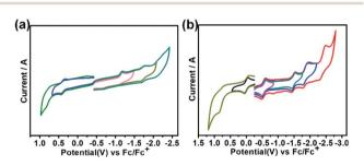
Fig. 4 Cyclic voltammogram of (a) Th@ $C_{3v}$ (8)- $C_{82}$ Ad(I) and (b) U@ $C_{2v}$ (9)- $C_{82}$ (I) in o-dichlorobenzene (0.05 M (n-Bu) $_4$ NPF $_6$ ; scan rate 100 mV s $^{-1}$  for CV).
