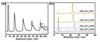
Fig. 2 (a) Recycling HPLC profile for the separation of  $U@C_{2V}(9)-C_{82}Ad(II)$ ,  $U@C_{2V}(9)-C_{82}Ad(II)$ ,  $U@C_{2V}(9)-C_{82}Ad(III)$  and  $U@C_{2V}(9)-C_{82}Ad(III)$  and  $U@C_{2V}(9)-C_{82}Ad(III)$  and  $U@C_{2V}(9)-C_{82}Ad(III)$  and  $U@C_{2V}(9)-C_{82}Ad(III)$  and  $U@C_{2V}(9)-C_{82}Ad(IIV)$ . HPLC conditions: Buckyprep column (10 mm  $\times$  250 mm); flow rate, 4 mL min<sup>-1</sup>; toluene as the mobile phase; wavelength 310 nm.
