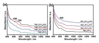
Fig. 3 UV-vis-NIR absorption spectra of (a) Th@ $C_{3v}(8)$ - $C_{82}$  and Th@ $C_{3v}(8)$ - $C_{82}$ Ad(I, II, III) and (b) U@ $C_{2v}(9)$ - $C_{82}$ and U@ $C_{2v}(9)$ - $C_{82}$ Ad(I, II, III) in CS<sub>2</sub>.
