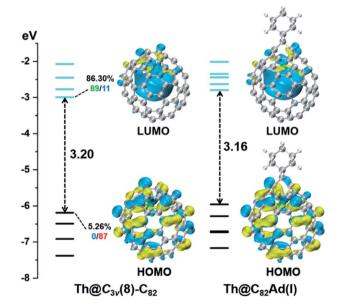
Fig. 9 Frontier molecular orbitals of  $Th@C_{3v}(8)-C_{82}$  and  $Th@C_{3v}(8)-C_{82}Ad(I)$  (occupied: black; unoccupied: cyan). For selected orbitals, the participation (%) of the Th AOs is first given, followed by two numbers showing the % contribution of the Th-5f (red), -6d (blue), or -7s (green) AOs to this metal hybrid orbital.
