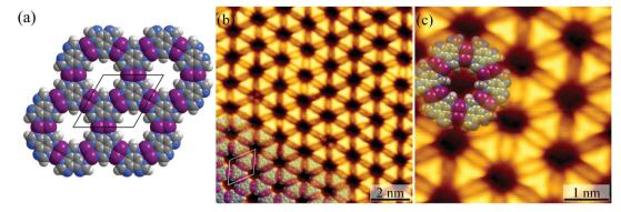
Fig. 3 (a) MM simulated structure of [Ag<sub>3</sub>btim]. (b) The large-scale (U = 1.6 V, I = 100 pA) and (c) high-resolution (U = 0.08 V, I = 1.54 nA) STM image of [Ag<sub>3</sub>(btim)] on Ag(111) surfaces. The unit cell is indicated in black/white in (a)/(b). Molecular models are superimposed on the respective image.
