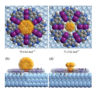
Fig. 5 DFT simulated primary host–guest structures on Ag(111) supported [Ag<sub>3</sub>(btim)] networks. (a and b)  $C_{60}$ . (c and d) Fe(Cp)<sub>2</sub>. (a and c) Top views. (b and d) Side views.
