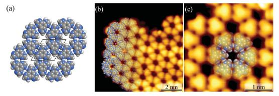
Fig. 2 (a) The 2D hydrogen-bonded network in  $H_3$ btim bulk crystals. (b) The large-scale (U = -0.2 V, I = 1 nA) and (c) high-resolution (U = -0.6 V, I = 100 pA) STM image of  $H_3$ btim molecules on Au(111) surfaces. The unit cell is indicated in black/white in (a)/(b). Molecular models are superimposed on the respective image.
