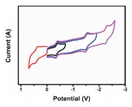
Fig. 8 Cyclic voltammogram of  $U_2N@/_h(7)-C_{80}$  in  $(n-Bu)_4NPF_6/1,2-dichlorobenzene.$
