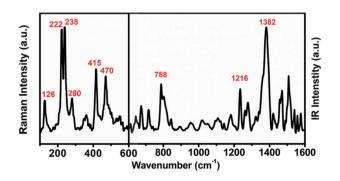
Fig. 3 Raman (left, up to 600 cm  $^{-1}$ ) and IR (right, from 600 to 1600 cm  $^{-1}$ ) spectra of U<sub>2</sub>N@ $I_{\rm h}$ (7)-C80.
