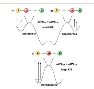
Fig. 2 The size of the KIE can be an indicator of the position of the transition state<sup>12</sup> (image reproduced from ref. 11). (a) For an early TS, the difference in ZPE between the TS and A is small, and a small KIE is obtained. (b) For a late TS, the difference in ZPE between the TS and B is small, and a small KIE is obtained. (c) For a symmetrical TS, where the H or D atom is fully dissociated, the KIE is largest.
