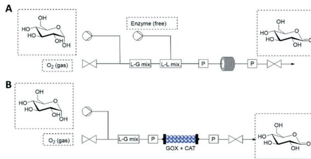
Fig. 6 Flow biocatalysis using pressurized reactors for the O<sub>2</sub> supply. (A) Free enzymes. (B) Packed-bed reactor with co-immobilized enzymes (GOX: glucose oxidase; CAT: catalase).
