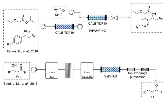
**Fig. 4** Schematic representation of chemoenzymatic dynamic resolution of benzylic amines developed by Farkas *et al.* and the fed-batch continuous flow hybrid process for the chemo enzymatic synthesis of 2-keto-3-deoxy sugar acids by Sperl *et al.*
