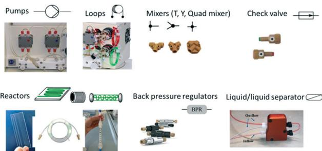
Fig. 2 Flow equipment and representation.
