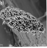
Fig. 1 SEM micrographs showing the change in the size of the microchannels before and after the modification. (a) Natural henequen fiber (b) henequen fiber modified with copper phthalocyanine.
