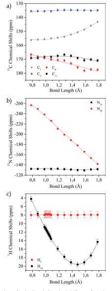
Fig. 4 Variation of calculated chemical shift as a function of  $N_{10}-H_{10}$  distance for different nuclei. (a)  $^{13}$ C, (b)  $^{15}$ N and (c)  $^{1}$ H.
