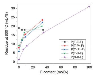
Fig. 7 Influence of the molar content of F units on the residue after TGA at  $800\,^{\circ}\text{C}$ .
