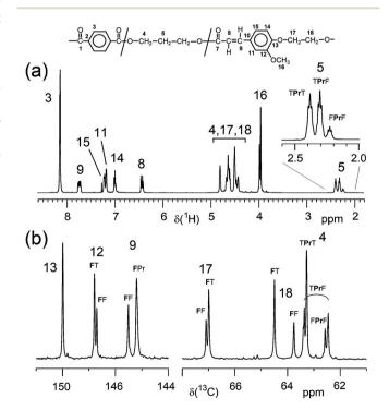
Fig. 2 (a) <sup>1</sup>H NMR spectrum and (b) two regions of the <sup>13</sup>C NMR spectrum of P(T-Pr-F)-7 (33.4 mol% F; solvent: CDCl<sub>3</sub>:TFA-d 4:1 v/v). Assignments to diad and triad signals are given.
