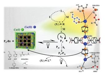
**Fig. 12** Proposed mechanism of ATRP polymerization catalyzed by the Cu(ii) MOF and the coordination structure of monomers and copper. Reproduced from ref. 125 with permission from the American Chemical Society, copyright 2017.
