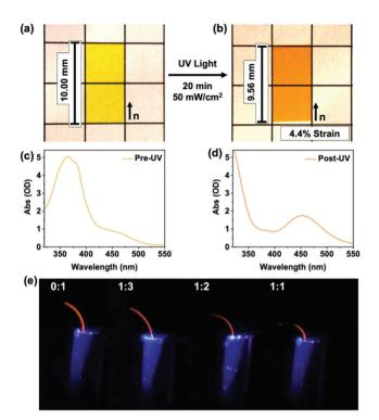
Fig. 6 Images of azobenzene-functionalized LCE (1:2 composition) (a) before and (b) after UV light exposure (365 nm, 20 min, 50 mW cm<sup>-2</sup>). UV-Vis spectra for film (c) before and (d) after UV exposure. (e) Monodomain azobenzene-functionalized LCE cantilevers (0.005 mm × 1 mm × 6 mm, increasing C6BAPE concentration from left to right) after 2 seconds of 365 nm light exposure (50 mW cm $^{-2}$ ).
