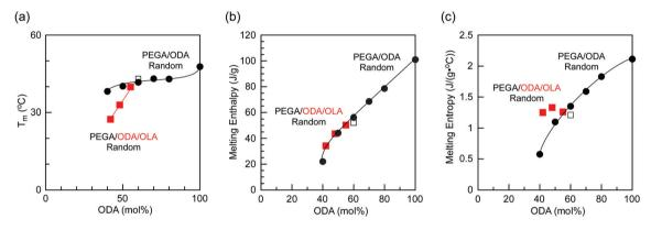
Fig. 5 (a) Melting temperatures and (b) enthalpy and (c) entropy of melting of octadecyl groups in PEGA/ODA/OLA random terpolymers (red squares: P2, P3, and P4) and PEGA/ODA random copolymers (black circles, 35 black open square: P1) as a function of the ODA content (mol%).
