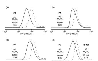
Fig. 2 SEC curves of (a) P2, (b) P4, (c) P7, their intermediates obtained at earlier conversion (dashed lines, PEGA/ODA + OLA conversion = (a) 16%/16%, (b) 20%/21%, and (c) 12%/12%), and (d) P9 and P9-1st (macroinitiator, dashed line).
