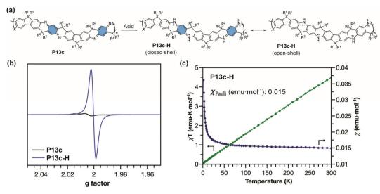
Fig. 14 (a) Structural representation of P13c and its acid-doped form P13c-H with closed-shell and open-shell resonance structures; (b) EPR spectra of P13c and P13c-H; (c)  $\chi$ -T and  $\chi$ T-T plots of P13c-H showing dominant Pauli paramagnetism. Reproduced from ref. 87 with permission from the Royal Society of Chemistry.
