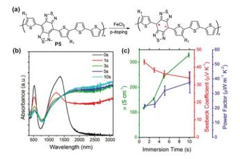
Fig. 13 (a) Structural representation of P5 before and after oxidative doping; (b) evolution of thin film UV-vis-NIR absorption spectra of P5 immersed in FeCl<sub>3</sub> solution as a function of time; (c) electrical conductivity, Seebeck coefficient, and power factor of P5 as a function of immersion doping time. Reproduced from ref. 94 with permission from the American Chemical Society.
