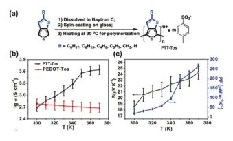
Fig. 12 (a) Synthesis and structural formula of PTT-Tos; (b) temperature-dependent conductivity of PTT-Tos compared with PEDOT-Tos; (c) temperature-dependent Seebeck coefficient and power factor of PTT-Tos. Reproduced from ref. 99 with permission from John Wiley and Sons.
