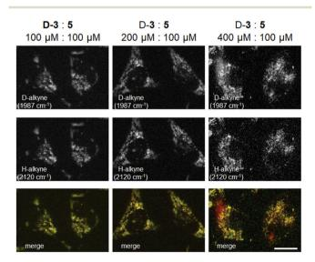
Fig. 5 Raman images of H-alkyne and D-alkyne signals in HeLa cells treated with D-3 and 5 at different dose ratios (1:1, 2:1, or 4:1) for 6 h. Images were obtained from the Raman intensity of the D-alkyne detected at 1987 cm<sup>-1</sup> and H-alkyne detected at 2120 cm<sup>-1</sup>. Two-color Raman images are the overlapped Raman images of the D-alkyne (red) and H-alkyne (green). Scale bars are 10 μm.
