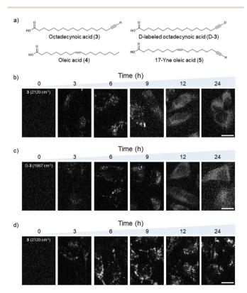
Fig. 3 (a) Structures of the C18 fatty acids. (b–d) Raman images of H-alkynes and D-alkynes in HeLa cells treated with 100  $\mu$ M C18 fatty acids at various times (0–24 h). Raman images obtained from the intensity of the C $\equiv$ C signal of (b) 3 detected at 2120 cm $^{-1}$ , (c) D-3 detected at 1987 cm $^{-1}$ , and (d) 5 detected at 2120 cm $^{-1}$ . Scale bars are 10  $\mu$ m.
